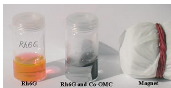
Figure 4. Rh6G aqueous solution (left) and after adsorption of the Rh6G on Co-OMC and separation of the dye loaded Co-OMC by a magnet (right).
